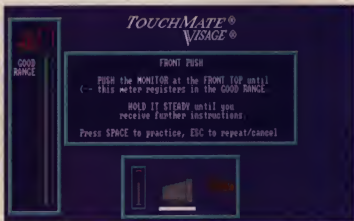
The calibration program in the TouchMate Control Panel lets TouchMate compensate for vibrations that may affect its ability to measure where the monitor is touched.
